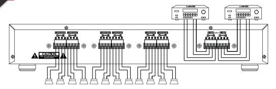
Insert your receiver/amplifier's positive (+) wires into the positive terminals, and negative (-) wires in the negative terminals.
