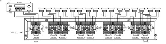
Press open the AMP terminals on the control center, then insert your receiver/amplifier's positive (+) wires into the positive (red) terminals, and negative (-) wires in the nagative (black) terminals. Then press the tabs to close them.
