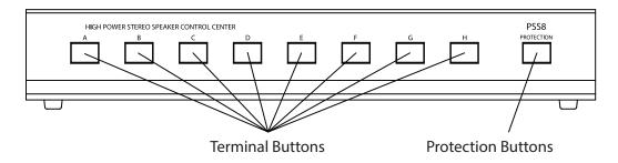
The control center lets you use one to eight sets of speakers at a time, and is designed to operate with a stereo receiver/amplifier that has a maximum of 100 watts per channel, and with speaker systems that have a minimum impedance of 8 ohms (see "Impedance Chart" on page 5)
