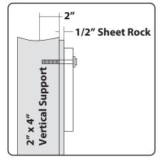
**Step #4:** Drill proper mounting hole (smaller than outer thread diameter of your lag bolts) through wall into wood studs or concrete block. Hole depth should be properly drilled so that your lag bolt can go through the sheet rock and 2" into the stud.
