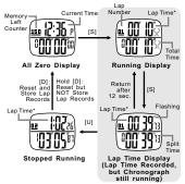
\*NOTE: The Lap Time within the first hour will be displayed as "Minutes, Seconds, 1/100 second". After then, it will be "Hours, Minutes, Seconds".
