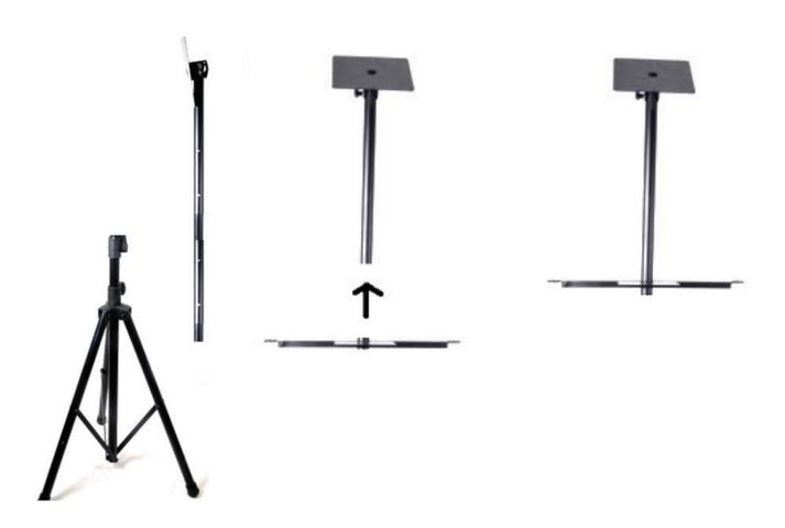
Insert back the top tube into the base tripod then start to assemble the TV/monitor as the above Adjust the height and angle you need and tighten the knobs to fix the height and angle. You can mount your TV box or other device on the small platform, you can use the included glued Velcro to prevent the device from sliding off. You can mount the microphone on the ring in the end of the cross bar or you can hang your headphone one the bar.
