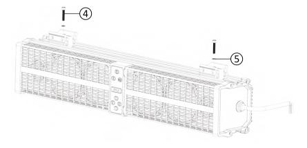
2. Align the screw holes at the bottom of the clamps with the positioning holes that have been made in the slider and lock the M5X24mm screws and M5 spring washers to fix the clamps.
