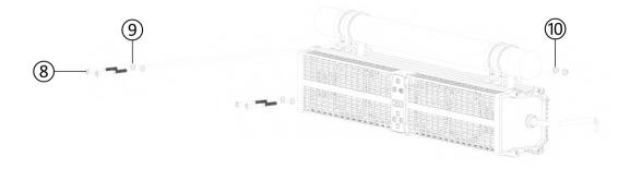
5. Use M6X60mm screws and M6 spring washers to pass through the aluminum ring and the base and the M6 non-slip nut at the back to fix the aluminum ring on the base as shown in the figure. Each nut should be installed in the hexagonal groove.
