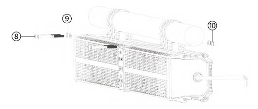
5. Use M6X60mm screws and M6 spring washers to pass through the aluminum ring and the base and the M6 non-slip nut at the back to fix the aluminum ring on the base as shown in the figure. Each nut should be installed in the hexagonal groove.
