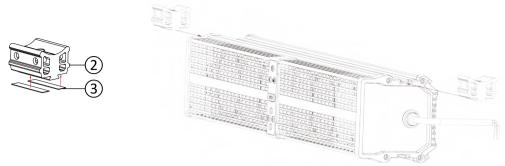
1. Stick the 45X10X0.5mm non-slip rubber strips (2 pieces) on the bottom of the clamps, then insert them into the slider.
