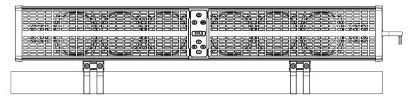
7. The installation steps of the aluminum ring below are the same as above, after complete installation, the PWPSB3202 will be above the cage bar as shown in the figure.
