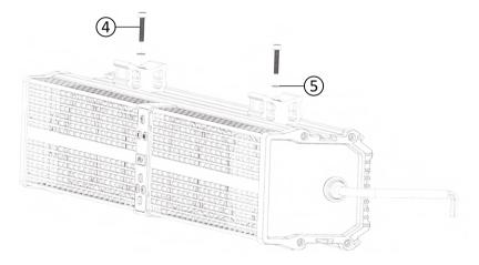
2. Align the screw holes at the bottom of the clamps with the positioning holes that have been made in the slider, and lock the M5X24mm screws and M5 spring washers to fix the clamps.
