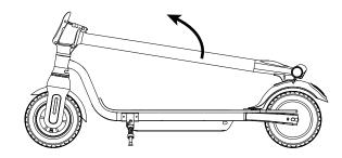
2. Get the long pole stand up, then pull up the folding wrench towards the upright pole and force it to stay close to upright pole
