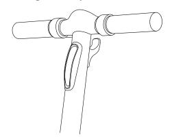
When the scooter is on, press (%) twice in short time to turn on the front light; When the scooter is on, press  $(^{\circ}\!\!/_{\!\!\!a})$  twice in short time to turn off the front light.
