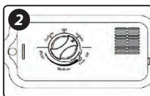
2 Turn Inflate/Deflate Switch clockwise to "Inflate" position to turn on Setup Pump and inflate air bed. Setup Pump will automatically turn off upon reaching selected firmness level and Inflate/Deflate Switch will automatically return to "Off" position.
