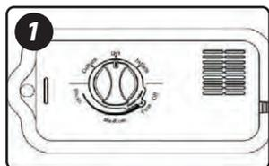
1 Constant Comfort Pump is a fully automatic pressure maintenance pump that is designed to operate silently so that it will not disturb your sleep when it automatically turns on to re-inflate. Pump will automatically turn on when air pressure inside air bed drops below a predetermined low pressure level. Pump will automatically turn off upon reaching selected firmness level (firmness determined through adjusting the Comfort Adjust Dial).
