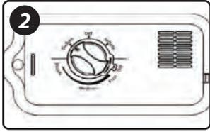
Turn Inflate/Deflate Switch counter clockwise to "Deflate" position for complete air removal. Upon complete air removal, Setup Pump will automatically turn off and Inflate/Deflate Switch will automatically return to "Off" position. Place power cord into Cord Storage Pocket for storage.
