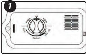
Turn Comfort Adjust Dial to "Off" position so Constant Comfort Pump will not automatically turn on.
