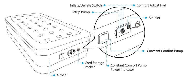
**SETUP OPERATIONS** (Before inflating, Plug into AC Power outlet.)
