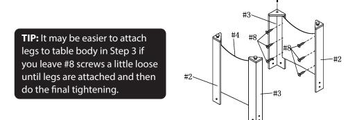
3. Attach assembled LEGS to TABLE BODY #1 with BOLT #6 and FLAT WASHER #7. **Note:** The table is assembled upside down.
