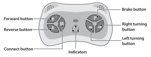
The remote control has precedence over foot pedal operation. (The foot pedal won't work while you operate the Remote Controller)
