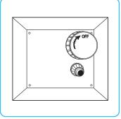
Check that the control knob for the gas supply system is turned to the "OFF" position before starting any assembly.
