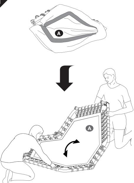
• Place Trampoline **A** on the ground and press it downwards into a flat position. Insert D-shape safety pin J into the fold at one end of the trampoline A entirely.
