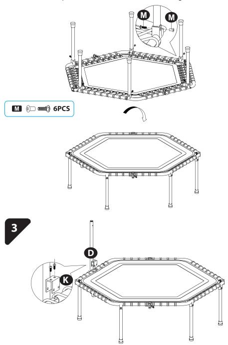
• Install grab pole **D** in the flattening place on the trampoline **A** with **G** and **K**.
