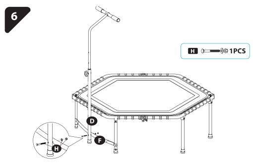
• First to attach cross bar **F** and grab pole **D** with **H**, then attach the ends of cross bar F with two feet B2 with K.
