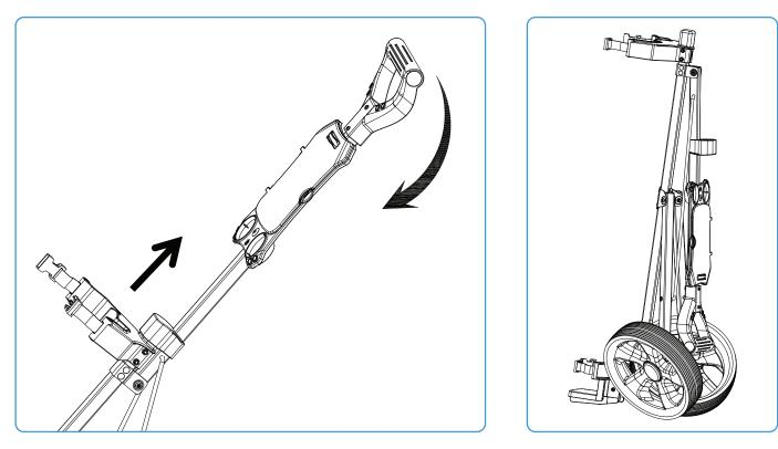
Move the slide lock toward upper and fold the handle as Fig. 5.
