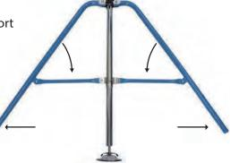
**3.** Layout and align the Main Support Poles 3 and Bottom Stabilizer Bars 4 like the diagram.
