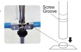
**6.** Finally, adjust the bottom of both Main Support Poles ③ to the point of where it is just barely above the surface.
