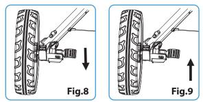
Push on the brake pedal to stop the rear wheel and pull off to release as in Fig.8 and 9.
