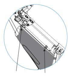
Point 2, Fixed the second velcro strap on the lower connecting rod, and only fix the velcro, so it can slide down and up when folding, do not fixed tightly, otherwise, it will affect folding the trolley. Point 3 & 4, Fixed velcro strap on the 2 holes leg frame, then pull the elastic strap and click into Point 5 & 6 on the 2 holes leg frame.
