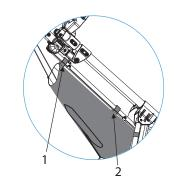
**Point 1, First step:** Fixed the velcro strap on the connecting rod, upper the plastic. Check the two sides elastic strap the same length.
