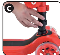
Pull the fixing sleeve upward as shown in Figure B & C.
