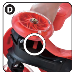
Press Red Switch with one hand and using the other hand to pull handlebar to separate the Handlebar and Scooters body as shown in Figure D.
