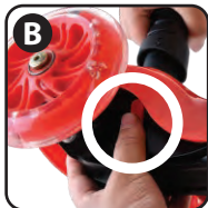
Press the red button, insert the sleeve and handlebar into the scooter
