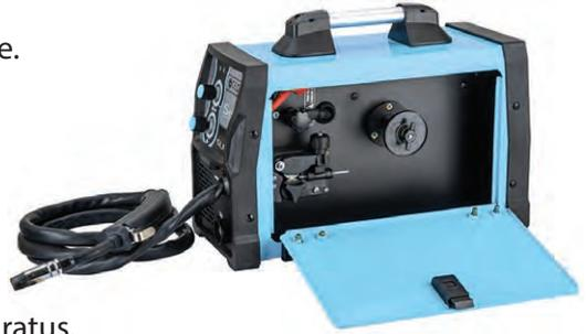
**Notice: if the pressure is too high, it will damage the wire; if the pressure is too low, the feed gear will slip, wire will not work properly.**
