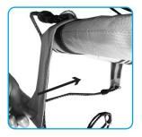
**13.** After the bolt assembling, and cover the velcro belt, and repeat 3 times on other 3 bolts.
