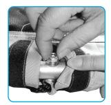
**11.** Tight it with screw nut, do not forget the washer.
