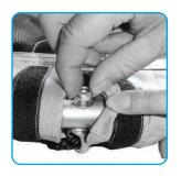
**11.** Tight it with screw nut, do not forget the washer.
