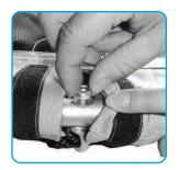
**11.** Tighten it with screw nut, do not forget the washer.
