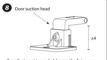
If readjustment is needed, loosen the fixing screw, the floor suction head can be adjusted by 4mm
