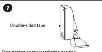
First, determine the installation position. Clean installation position with a wet cloth then make it dry. Peel off the double-sided tape on the bottom surface of the door suction base.
