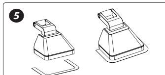
Peel off the tape, align the door suction head base with the position of 3M template and attach the door suction head to the floor. Peel off the 3M template tape after finish.
