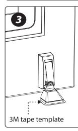
Stick the 3M tape template on the floor along the edge of the door suction base.
