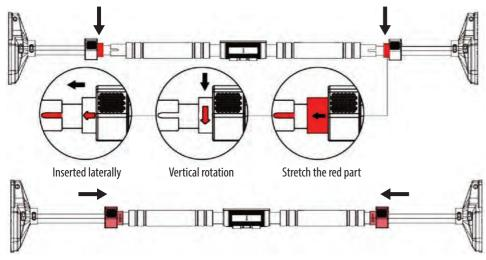
**Reminder:** After we receive the horizontal bar, if the lock and the pole are tight and the big foot pole is difficult to turn out, we must first loosen the locks on both sides.
